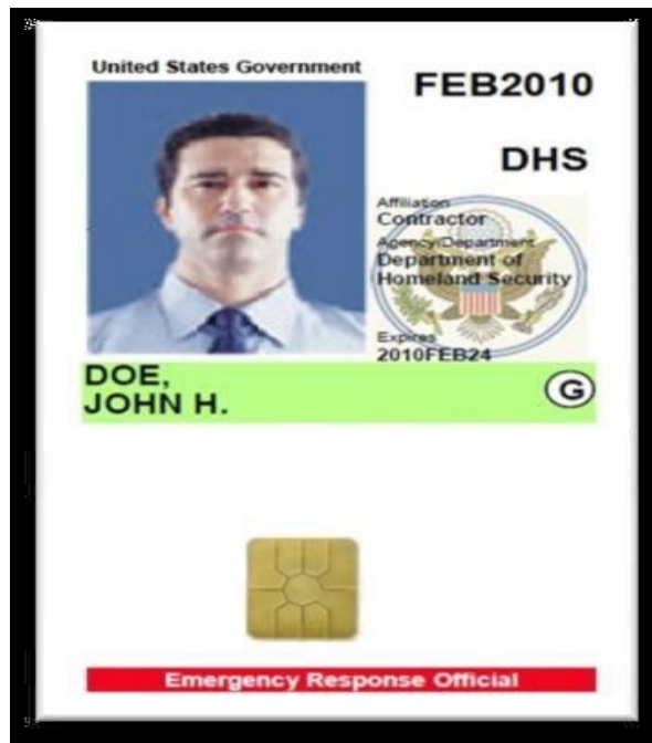
Figure 2 - A final component of an APL PACS is the employee's Personal Identity Verification (PIV) card.
